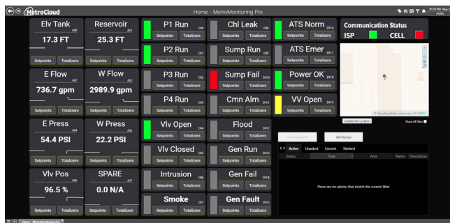
Metro Monitoring Pro interface via MetroCloud connected device.
