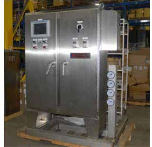
When potable water is used to provide seal water flow, it is important to address the need for back flow prevention. Many designers and public health authorities favor a physical air-gap/ break tank as a positive means of separating the water source from the process. Physical air gap type systems require a pumping system to re-pressurize the water for seal water service.
