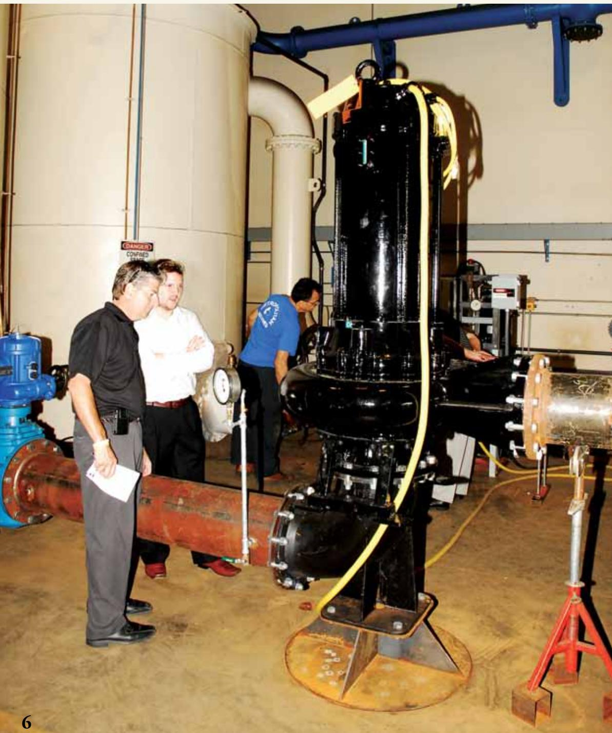
Metropolitan obliged and testing included performing both a flow test and a hydrostatic test on each of the three pumps in one day while the customer's consulting engineer was present to witness.
