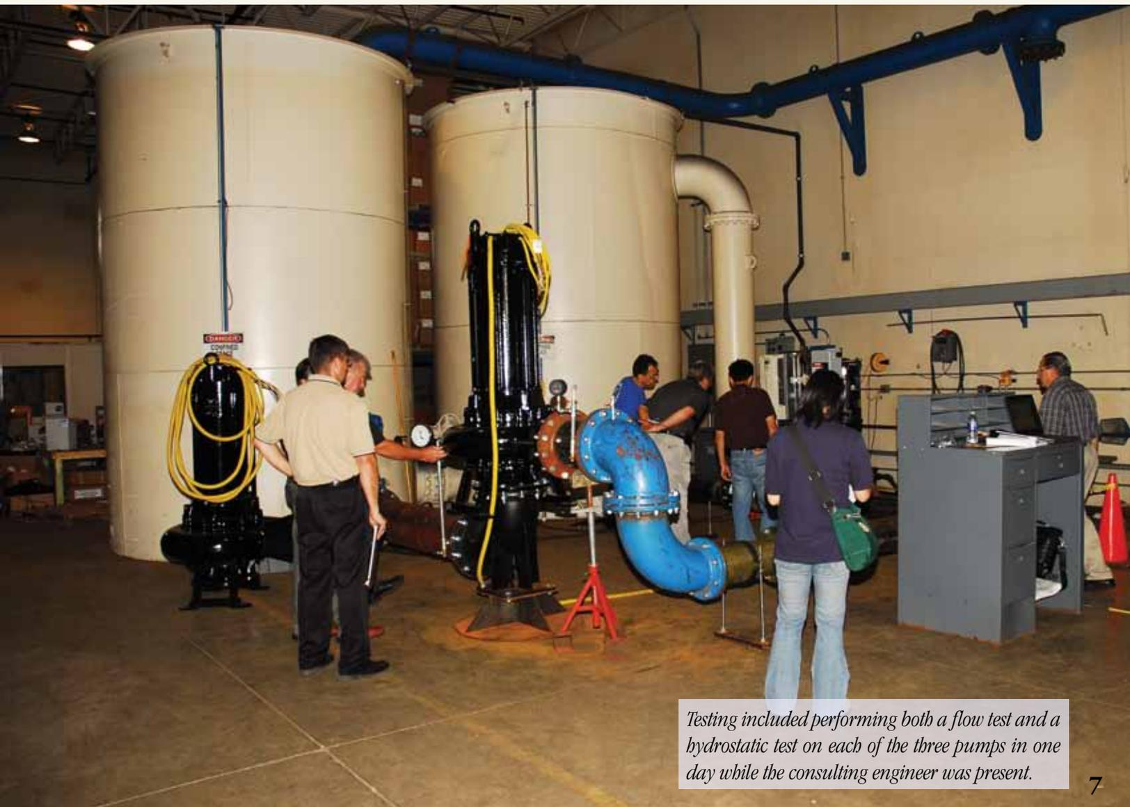
*Testing included performing both a flow test and a hydrostatic test on each of the three pumps in one day while the consulting engineer was present.*
